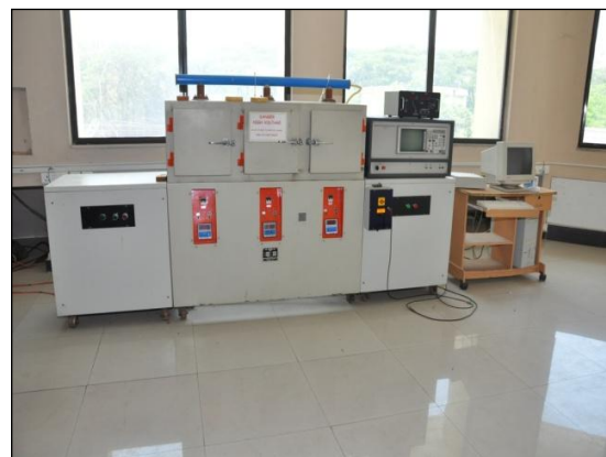
Accelerated ageing test set up for ZnO blocks.
