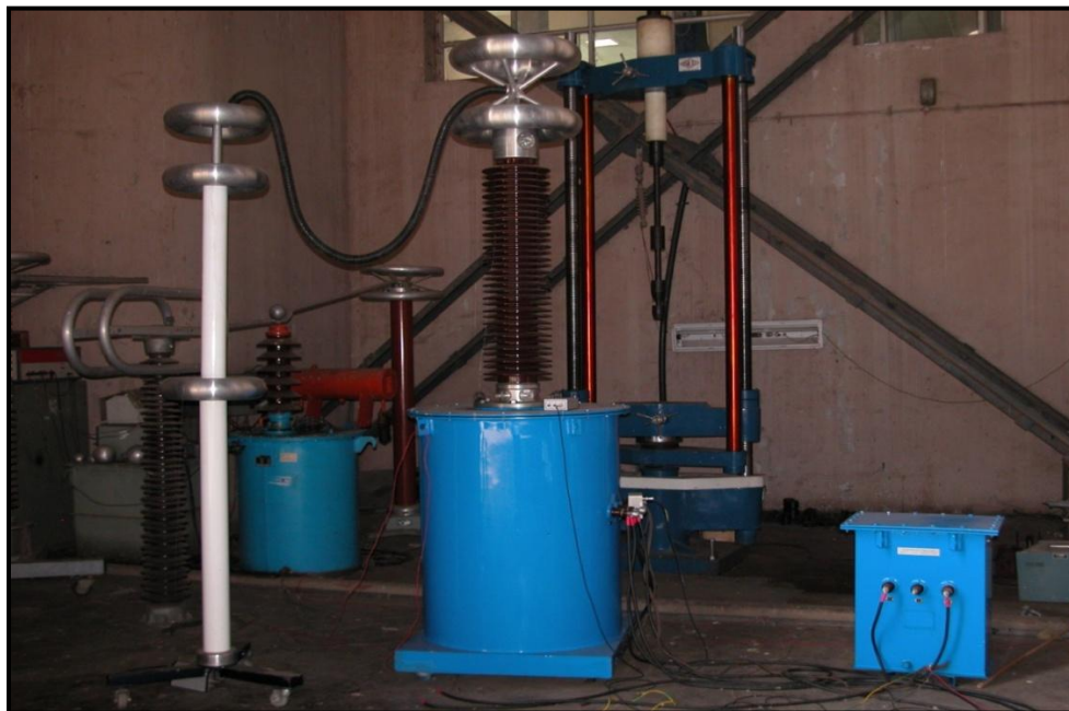
150kV, 300kVA Testing Transformer
