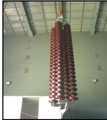
400 kV Quadra pole insulator string under pollution test
