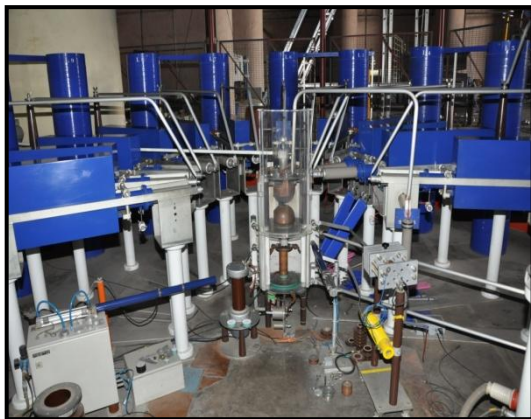
Impulse Current Generator 100 kV, 150 kJ
