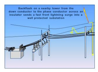
station. The studies include both switching surge analysis and lightning surge analysis. Even though stations are usually shielded, the lightning surge finds its way into a substation when there is a backflash on any incoming line. The resulting current levels in the station are quite low relative to direct strikes, but all that is needed to fail insulation is voltage and not current. (Index)
