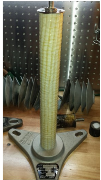
Figure 13 – Internal module of arrester 2153008505.
