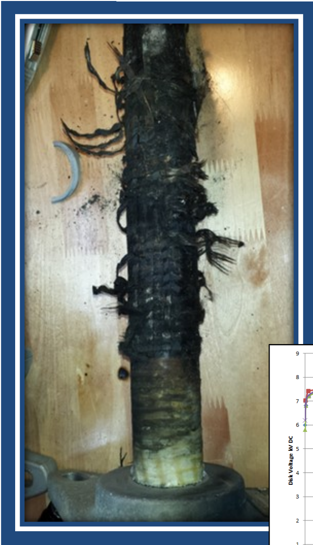
MOV Disk Fragments carry all the characteristics of the full disk if measured electrode to electrode
