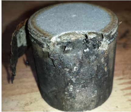
Figure 3 - Carbon and melted aluminum as a result of flashover.
