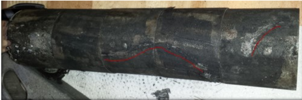
Figure 5 - Carbon on disks from failed arrester 21353008506. Red line traces tracking on side of disks.
