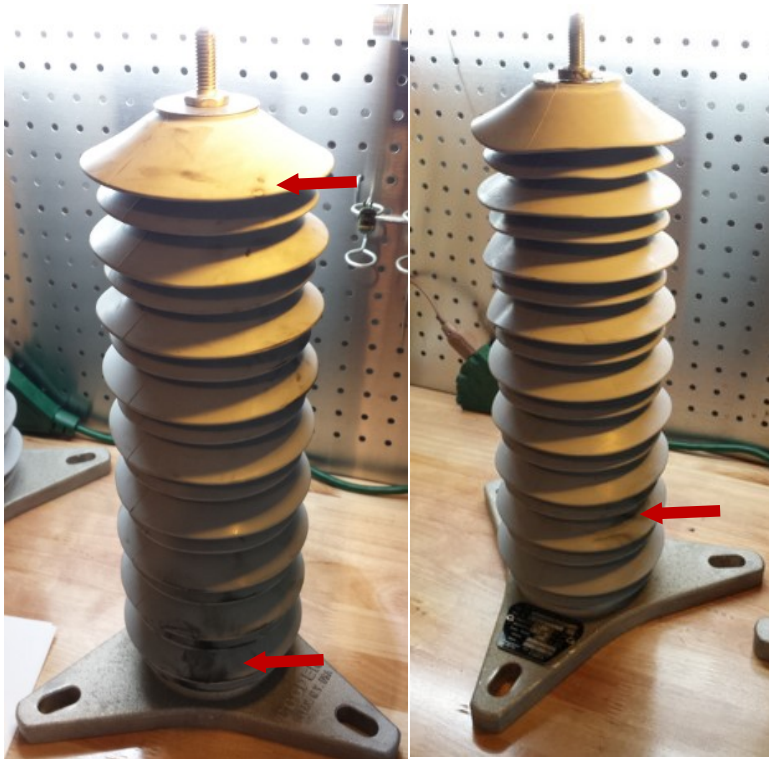
Figure 1 – Burn marks resulting from flashover on arresters 21353008504 (left) and 2153008505 (right).
