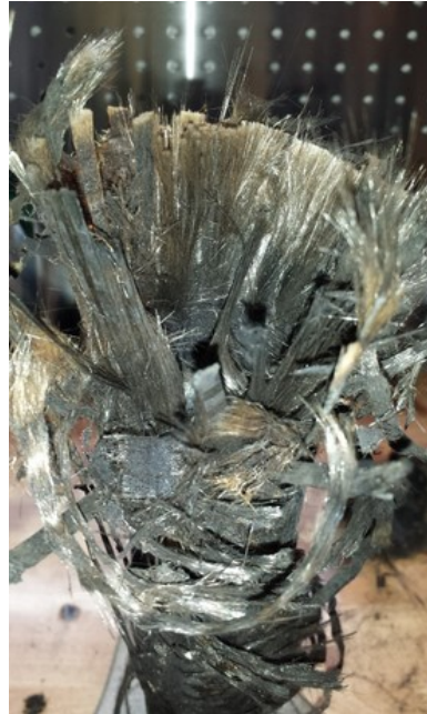
Figure 4 - Depolymerization of fiberglass wrap
