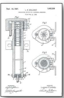
First Failed Arrester Indicator Patent (Filed 1922)
