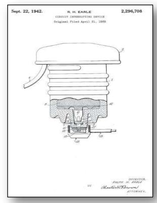
First Failed Arrester Disconnector Patent (Filed 1939)
