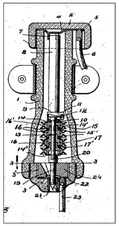
Figure 8 Early Expulsion Arrester from 1918 McFarlin Patent using hot moving air through the gap section to increase the arc length and resistance.
