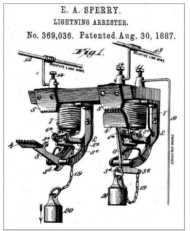
Figure 1 Early Power System Lightning Arrester. Gap between plates 4 and 5 opens up when follow current from the system activates the solenoid 7 allowing weight 20 to pull down and effectively increasing gap resistance.
