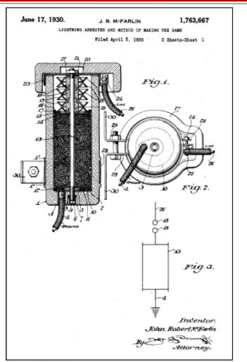
Figure 8 First Silicon Carbide Arrester Patent Filed in 1926 and Issued in 1930
