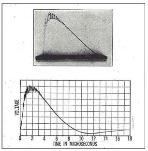
Figure 9 Ocillographic recordings as shown in the 1927 AIEE paper "The measurement of Surge Voltages on Transmission Lines Due to Lighting
