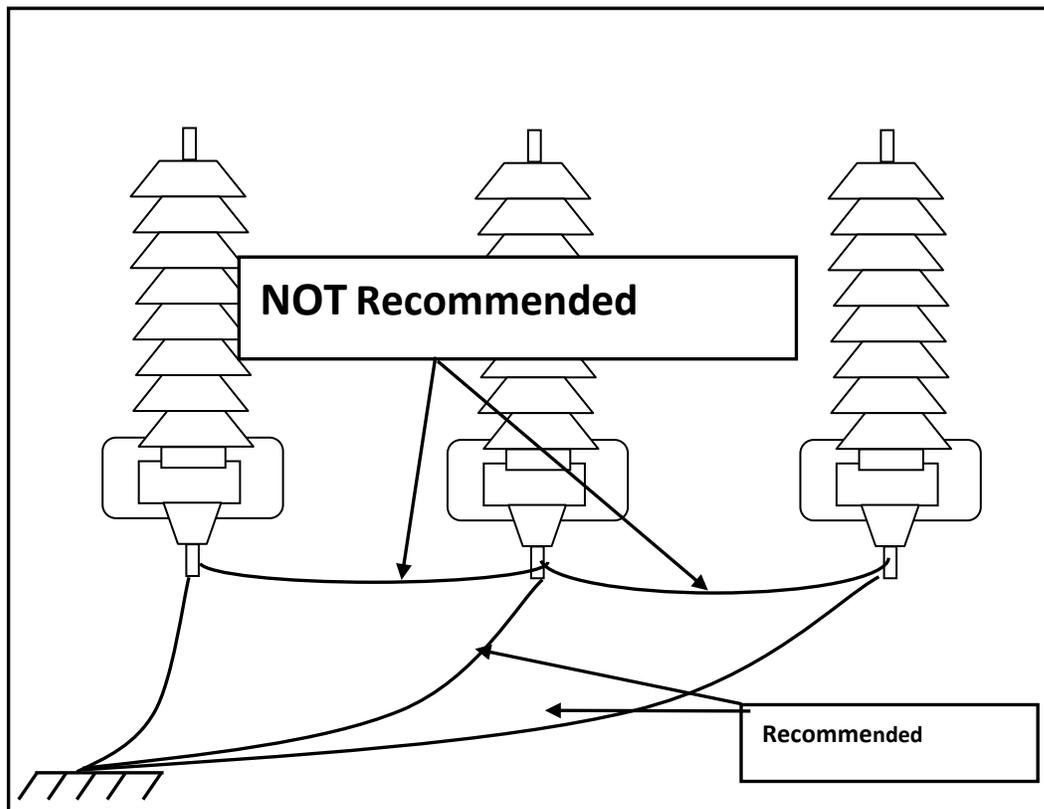
Figure 5 Recommended Lead Management for 3 phase parallel connection
