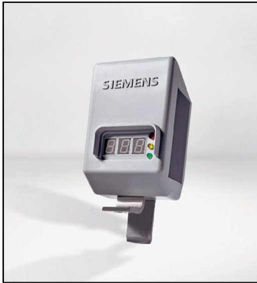
Figure 6 Siemens ACM (Arrester Condition Monitor) with advanced communications capabilities and 3rd harmonic evaluation of leakage current
