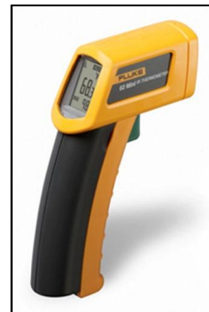
Figure 10 Infrared Thermometer A cost effective means of assessing the temperature of an arrester.
