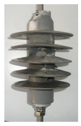
Figure 6 Acceptable Failure Mode
