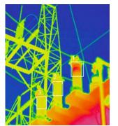
in time. It cannot show temperatures through time unless the camera has been recording it through time which is often an option. With regard to arresters, the only negative attribute of this test method is that it cannot be used if the arrester has been de-energized for more than a few minutes. Since it is not a standard piece of toolbox gear, sometimes the output is not readily available at the test site by non imaging personnel.
